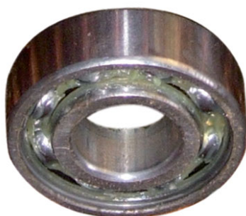
Fig. 12.16 : Ball bearings reduce friction
