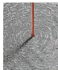
Figure 13.6 (a) A pattern of concentric circles indicating the field lines of a magnetic field around a straight conducting wire. The arrows in the circles show the direction of the field lines. (b) A close up of the pattern obtained.
